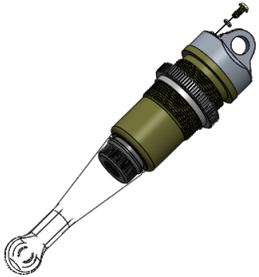
6. Finish reassembling shock with spring cup, shock spring and spring retainer (The soft spring is recommend as a great place to start). Now mount and adjust (with car body off) spring adjustment nut until drive shafts become level.
